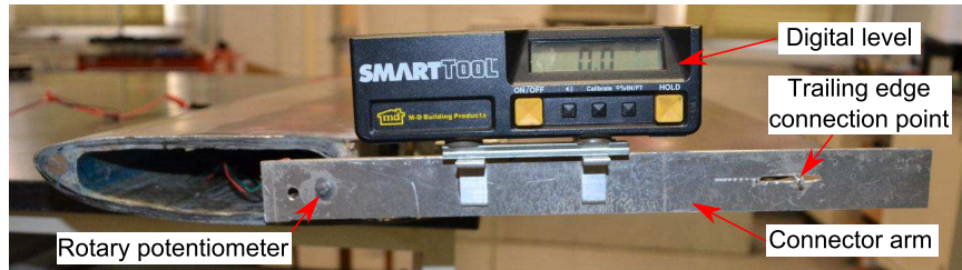
Figure 5.26. Front view of the camber sensor (installed on the prototype)
