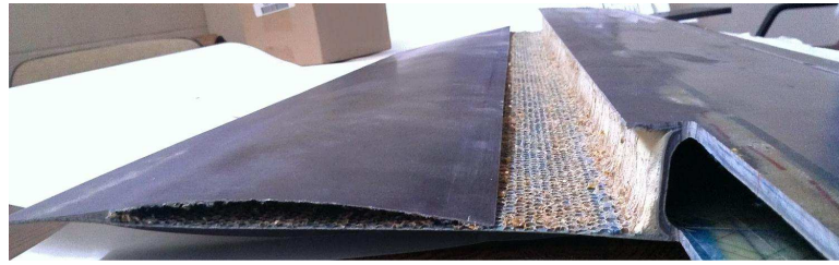
Figure 5.15. Exterior view of the blade skin aft of the D-spar web wall with the honeycomb removed
